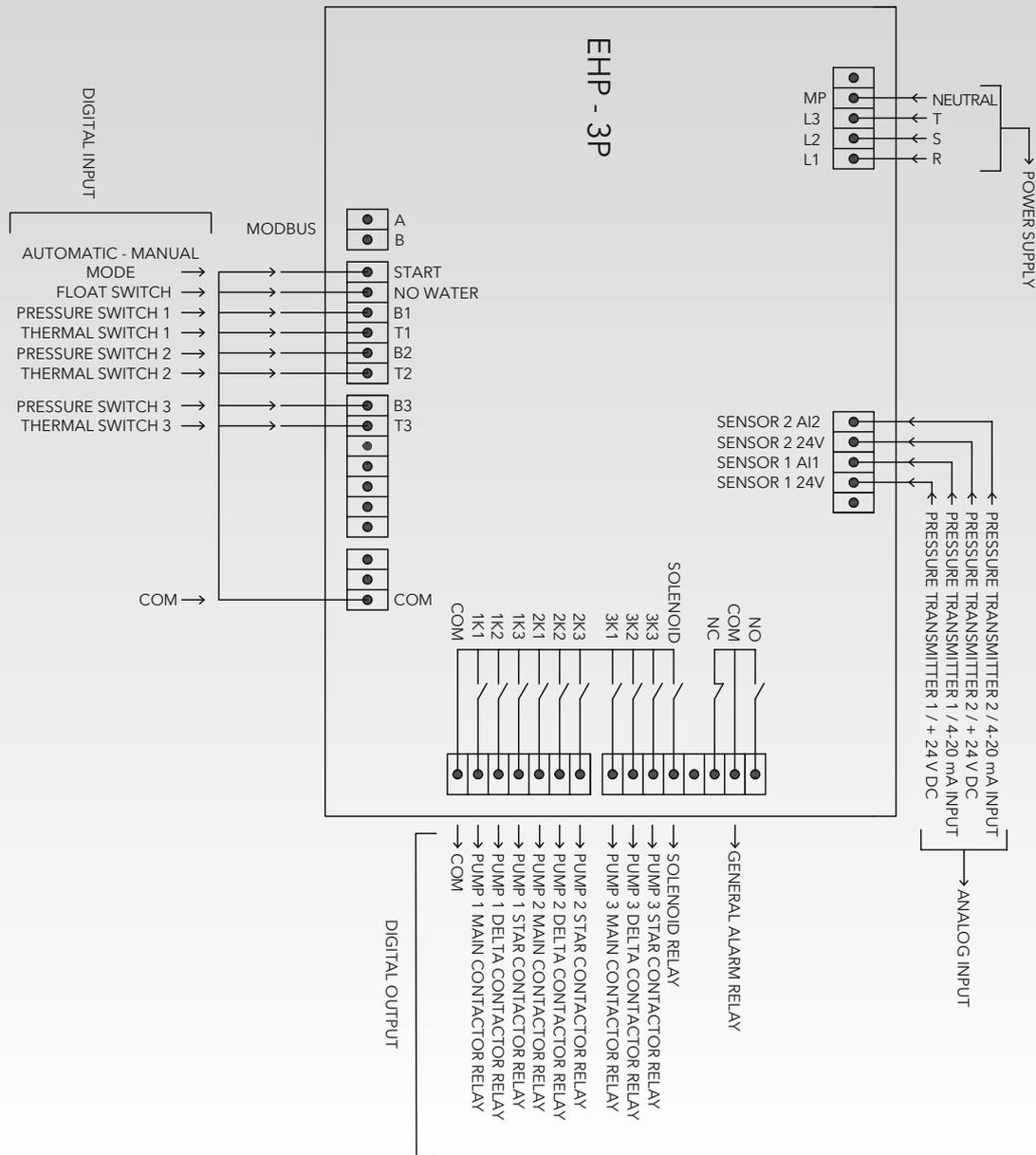
Figure 29. EHP-3P Pump Controller Terminal Descriptions
