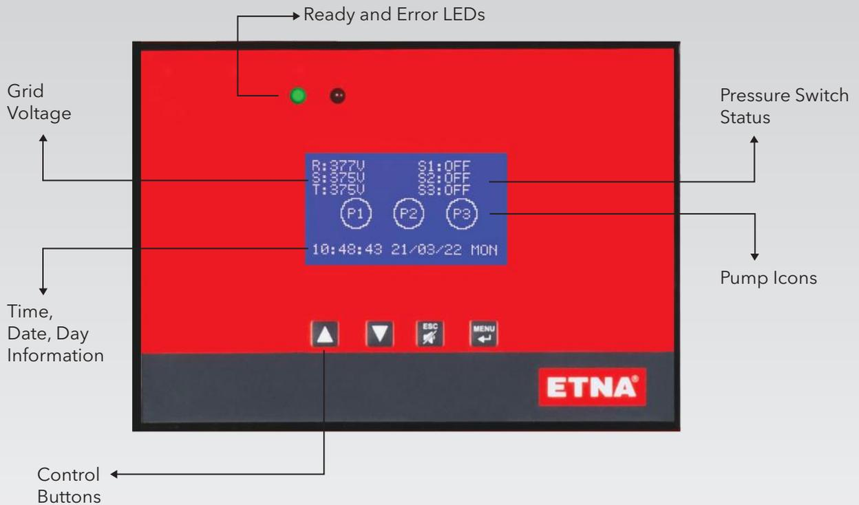
Figure 3: Pump Controller
