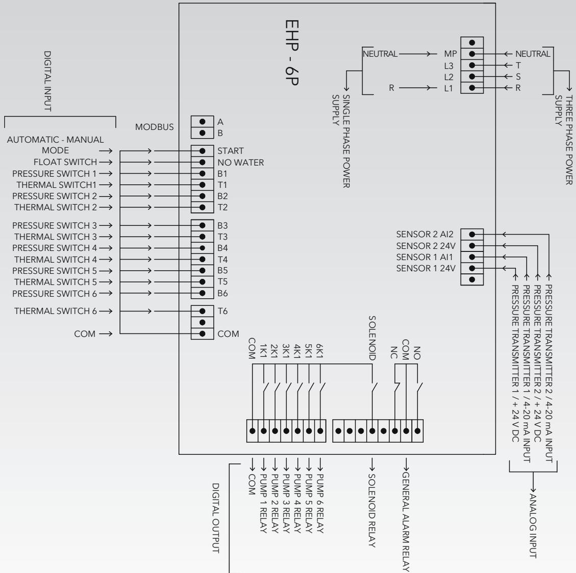
Figure 30. EHP-6P Pump Controller Terminal Descriptions
